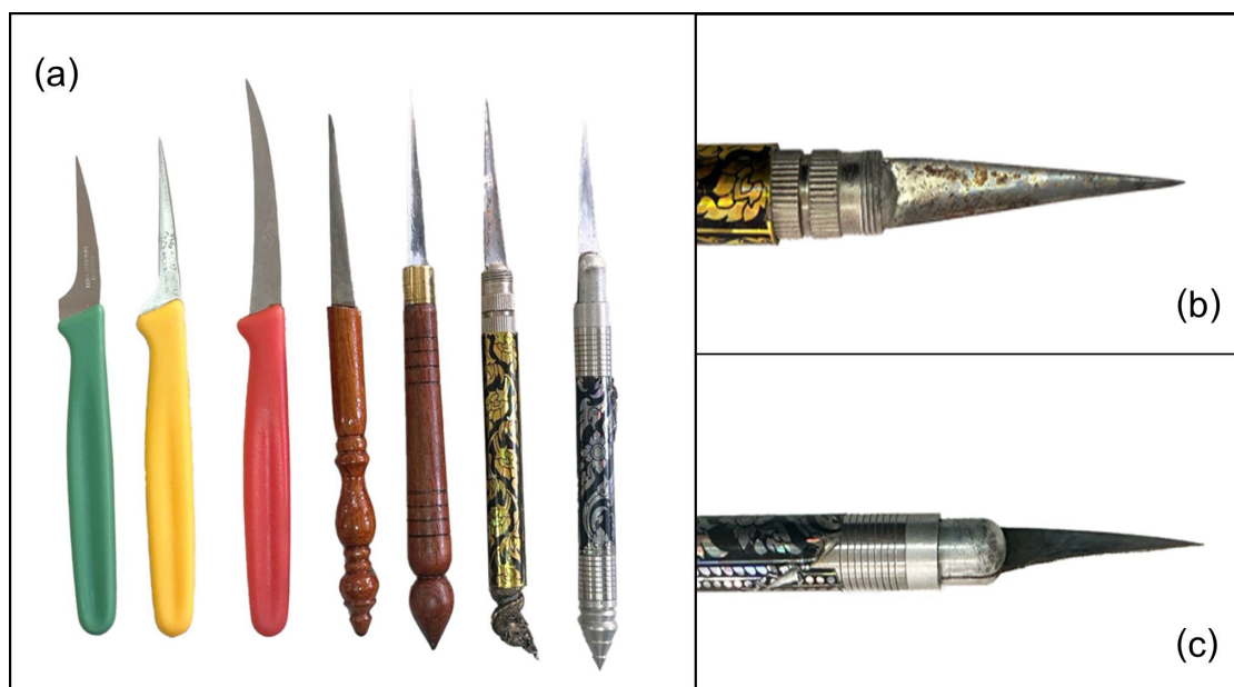
Figure 3 (a) The common types of carving knives available in the market (b) A rusted blade (c) Peeled-off Thai-pattern stickers
