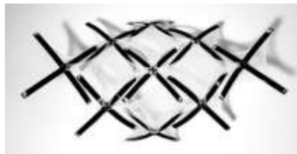
Figure 15: Experiment to Connect the Sub-Units within a Two-Layer Tensile Surface Structure
