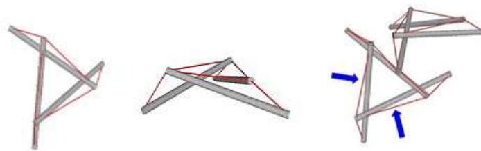
Figure 6: Tensegrity Sub-Unit Dome System
