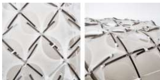
Figure 19: Double-layer Tensegrity structure model
