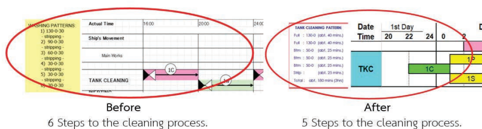
Figure 4 Comparison of tank cleaning patterns.
