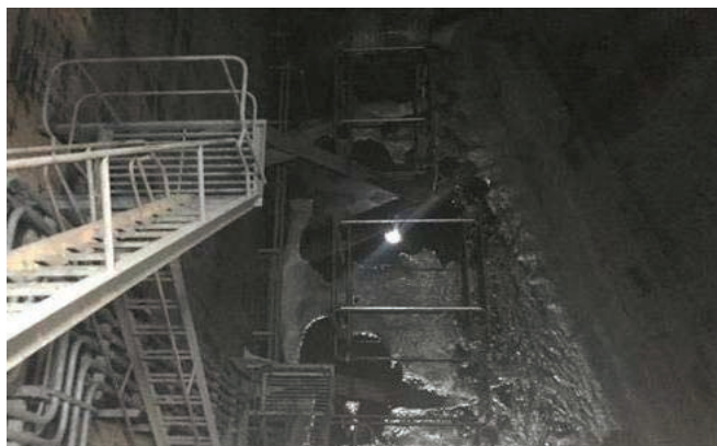
Figure 6 Sludge in the cargo tank
