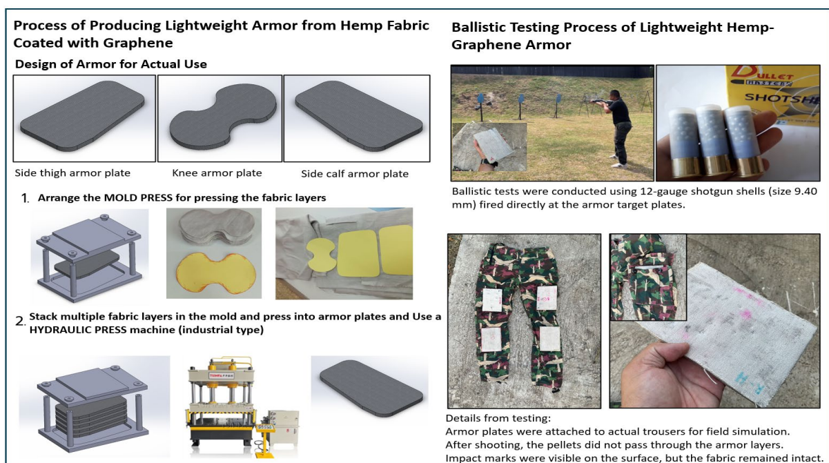
Figure 2 Prototype of graphene-coated hemp plates and ballistic testing results using 12-gauge shotgun
